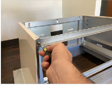
10. Remove the upper front panel support bracket with hardware and set aside.
