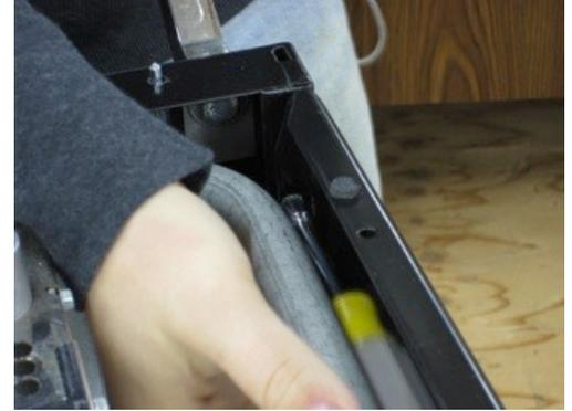
3. Remove the phillips screws along the top of the control panel and all the handle knobs across the front.
