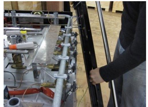
5. The control panel venting flange slides just under the flashing located under the valves when reinstalling the control panel. Mind the oven control shafts when reinstalling. Install in reverse order.
