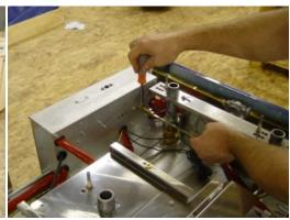
4. Remove electrical box top with attached safety switch and drape over back panel.
