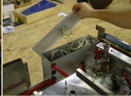
5. Remove both 7mm screws at each side. These screws are installed from the rear. These will be difficult to remove considering the back panel will be close to the wall. If a 7mm nut driver is too long, consider using a 7mm open end wrench or socket to loosen the screws.
