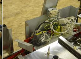
8. Loosen the screws holding the spark module in place and remove the module.
