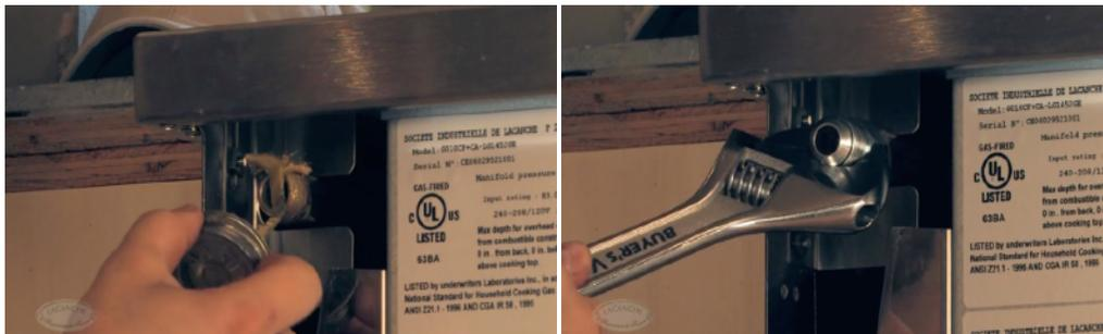
Now connect the flex line to the compression fittings. The compression fittings do not require compound sealant, but must be made tight enough to prevent fuel leakage. Use a wrench on each hex fitting to ensure tight seal.
