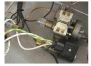
6. Inspect all wiring for fraying and breaks, especially at the spade connections on the terminal block, thermostat, selector switch, and 120v solenoid.
