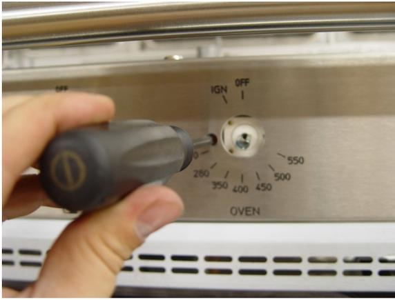
With a flathead screwdriver, turn the selector screw counter-clockwise all the way to the stop, labeled “N” for Natural Gas or clockwise to the stop, labeled “LP” for Liquid Propane.
