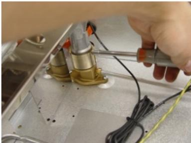
With a 7mm nutdriver, loosen the air collar and shift it up out of the way to get to the injector. Remove the injector with a 12mm wrench. Use the new washer supplied with the new injector.
