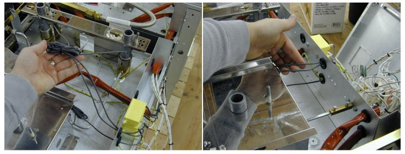
Loosen the square backing nuts with a pair of pliers or an adjustable wrench to release the module.
