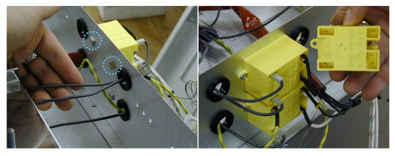
You may have to remove the electric oven knob shaft and all four 7mm hex screws to detach the front part of the electrical panel enough to remove the spark module screws.
